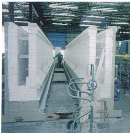
Prefabricated side wall sections of a sanitaryware tunnel kiln before shipping to the job site. BNZ 26-60 IFB is used on the hot face and BNZ 2300 HS IFB is used as back-up insulation.
