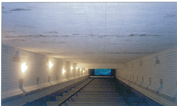
Looking into a 16 foot wide sanitaryware tunnel kiln lined with the specialty grade brick.
