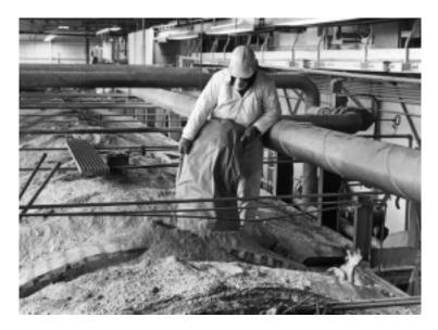
Materials' Blazelite insulating aggregates are formed by crushing large slabs of specially formulated low-density insulating material. The pulverization process is done with special equipment designed especially for this type of material.
