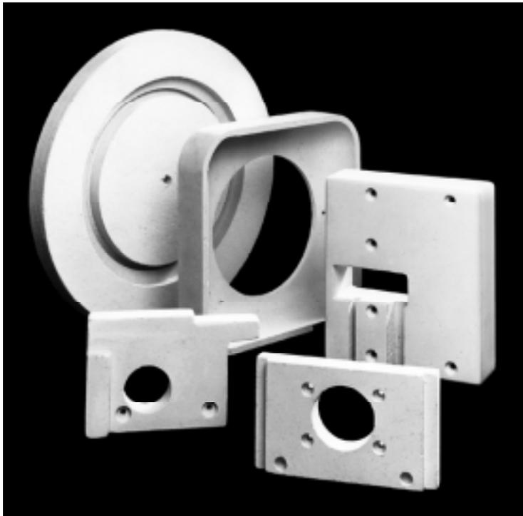
**M**arinite I structural insulation is a non-asbestos incombustible material manufactured in 4' x 8' panel form. These boards are designed to combine structural strength and high thermal insulating values in a variety of fireproofing and heat processing equipment applications. Formed from calcium silicate with inert fillers and reinforcing agents, Marinite I panels provide structure and insulation in a single, easily erected material.
